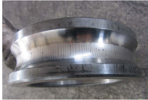
Fig. 17. Bearing fault on inner race in drive end of generator.
